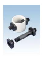
In order to join tube diffusers intended for square headers to 4-inch round headers there is a special connecting set available. Each set consists of 2 saddles and one connector threaded on both ends with 1" male threads. Other pipe dimensions and threading in preparation.
